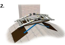
Carry up folded C.A.R.S unit and assemble platform and end frames in upside down position, as shown.
