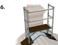
Fit two horizontal-rail braces onto the verticals of the frames. Ensure the hooks are inboard on the platform side.
