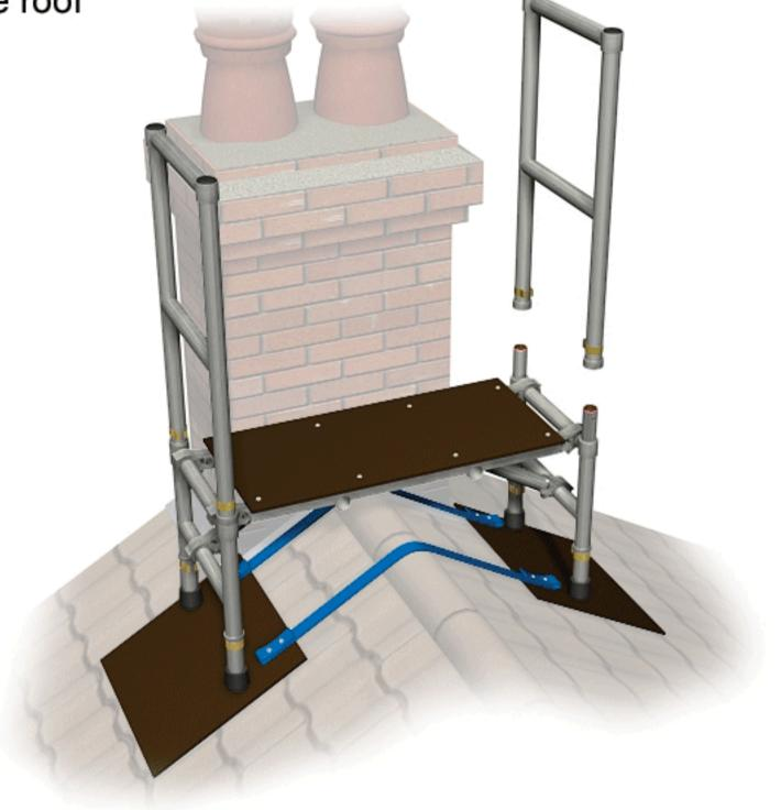
Turn the unit over and ensure the round rubber feet are seated evenly on the base boards. Ensure the platform is level. Use the telescopic legs to level the unit, for example, when roof pitches vary.
